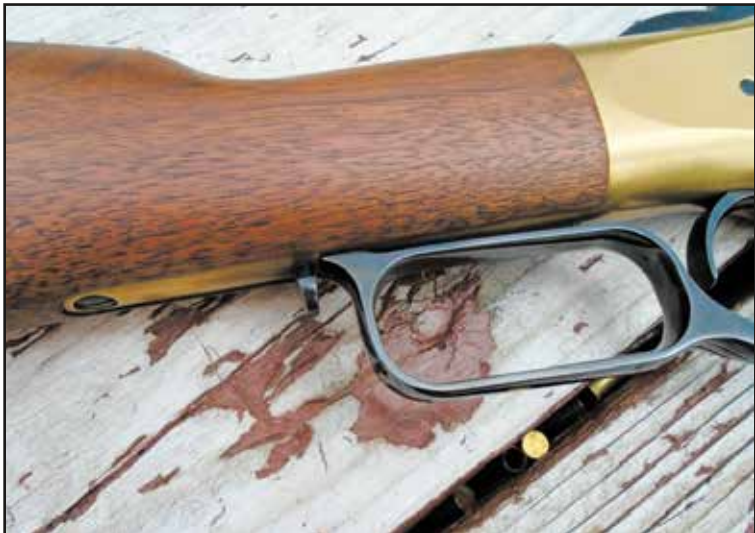
Like the original, the Winchester 1866 has a lever lock to keep it from opening when you don't want it to.
