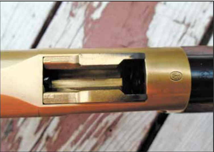
Empty shells are ejected out of the top of the receiver.
