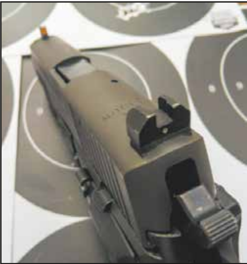
The XS F8 sights are more like traditional notch and post models but with a handful of speed optimization features.
