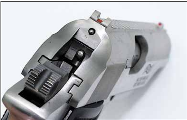
Top:The Walther PP .380 ACP Pistol has a loaded chamber indicator. Below: Walther PP .380 ACP Pistol's front sight.
