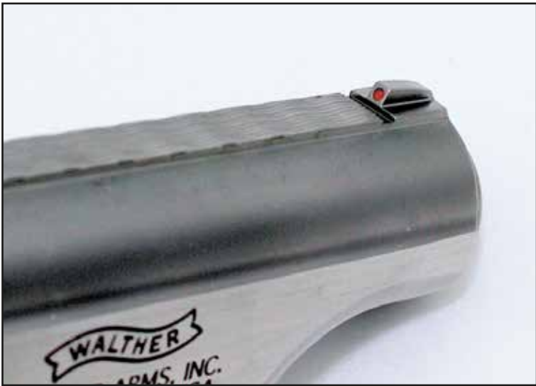
Top:The Walther PP .380 ACP Pistol has a loaded chamber indicator. Below: Walther PP .380 ACP Pistol's front sight.
