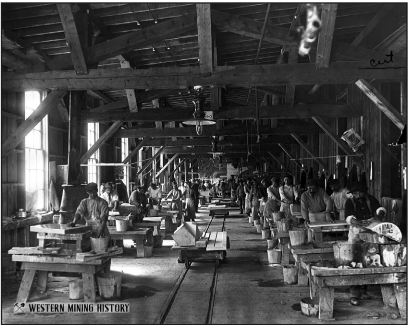
Workers hand polish marble slabs at the Yule Marble Co finishing mill
