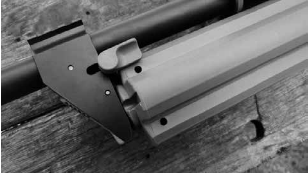
Flip these tabs up and the tube can be easily rotated.
