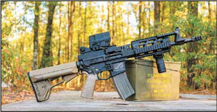
The FightLite MCR can feed from a standard M249 SAW belt or a STANAG magazine. IMG Jim Grant
