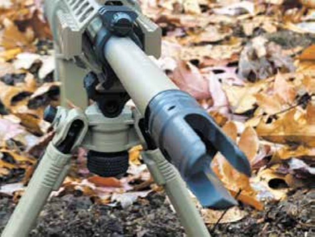
PSA Sabre AR-10 Muzzle and adjustable gas block
