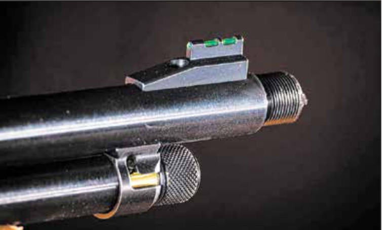
The Model X's green front sight contrasts perfectly against the rear orange. Also, note the threaded barrel – perfect for suppressors. IMG Jim Grant
