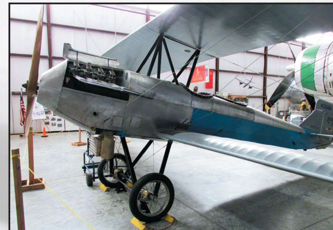
Side view of the Alexander EagleRock showing its rather delicate landing gear.
