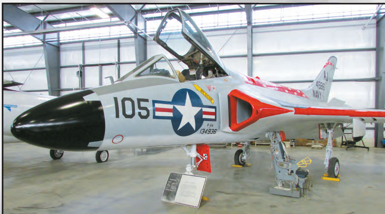
F-6 Skyray. 1956-64 USN carrier attack aircraft. Never used in combat. First Navy aircraft to exceed Mach 1 - over 700 mph. The SkyRay provided the basic design for the A4 Skyhawk.
