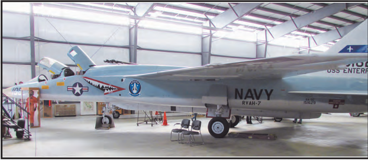
RA5C Vigilante Largest carrier based aircraft - 76 ft. long Supersonic 1300 mph NUKE bomb capability. Usual role was high altitude photo recon. 50,000+ ft Superceded by the SR-71 Blackbird.
