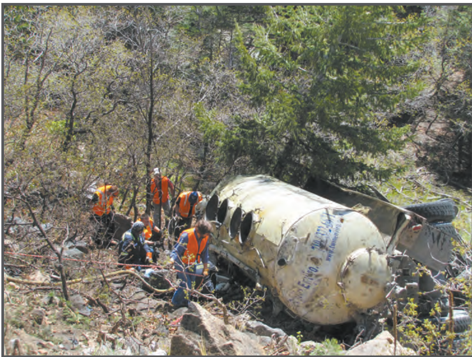
The recovery crew works to drain the tank and prepare to remove the wreckage.
