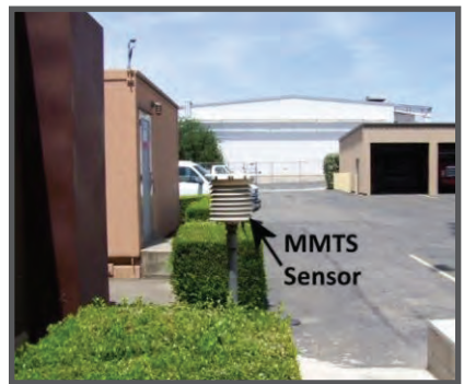
USHCN weather station in Marysville, Calif. is located next to an asphalt parking lot and near several air conditioning exhaust vents.(surfacestation.org)
